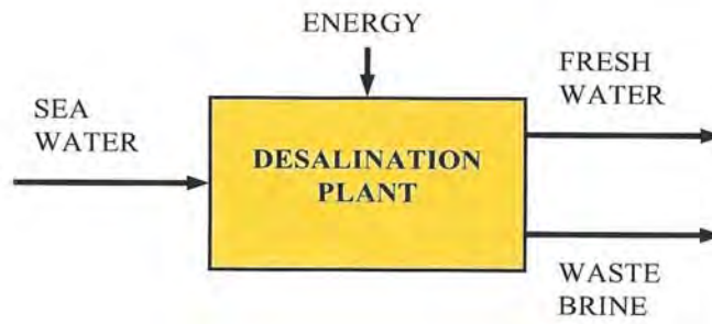
Figure 5: Basic principle of desalination.
